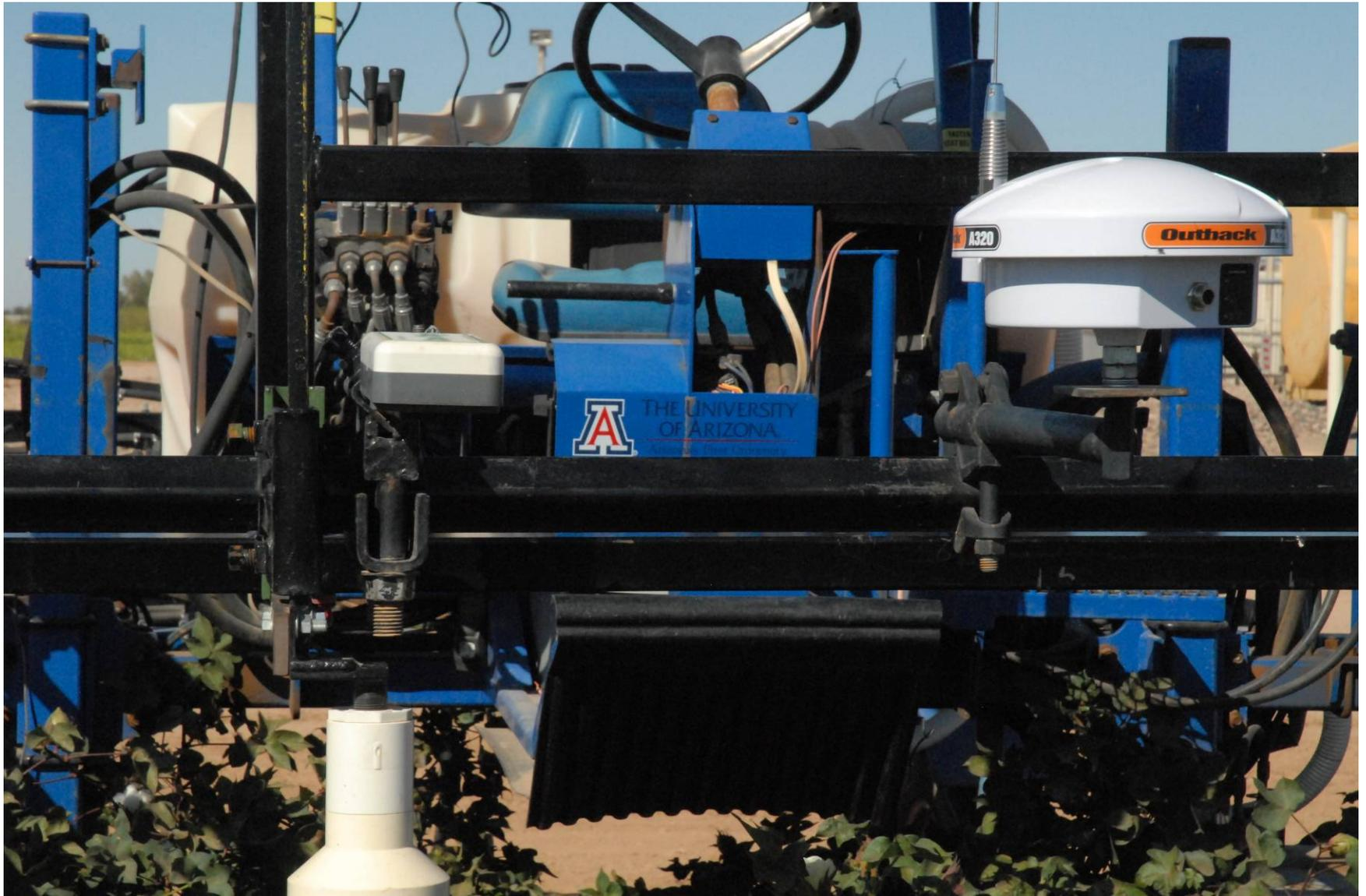
Sensor position – horizontal adjustment (rotation)
